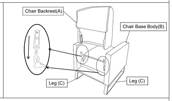
Chair Backrest(A)socket is aligned with the mounting position on the Chair Base Body(B), and the Chair Backrest(A) is firmly but gently pushed down until the Chair Backrest (A) is fully grooved and locked in place.
