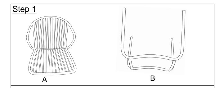
Unpack and place all parts on a clean, non-marring surface. Position the Leg Frame (B) resting on its front, as show in Pix B above.
