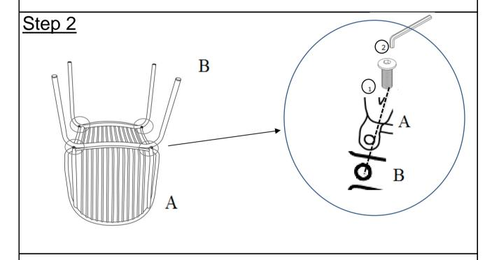
Attach the Leg Frame(B) to the Chair Seat(A) using Bolts(1) with Allen key(2). **Do not fully tighten Nuts.**
