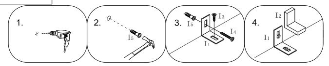
If it is a solid wall, please use expansion and self-tapping screws, if it is a wooden wall, only use self-tapping screws, please do not overtighten the screws
