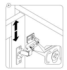
To adjust the gap from the door to the main frame turn the screw clockwise or anti-clockwise as needed.
