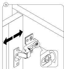
To adjust the door laterally adjust the screw as shown by turning clockwise or anti-clockwise.
