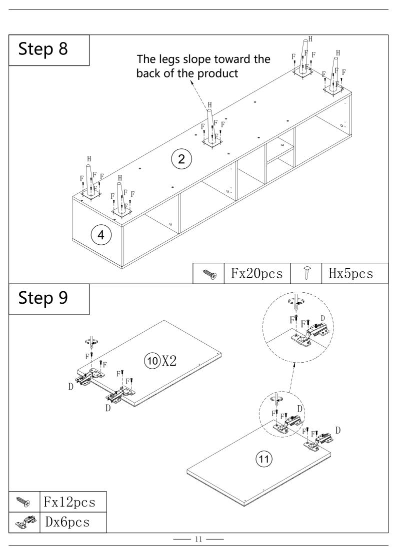
After the completion of step 8, the cabinet needs to be turned over180° to facilitate the installation of hardware G and F,It takes two people to flip and be safe!
