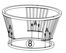
The finished product assembled in step 5 needs to be turned 180 degrees and fixed to part 8 with screw A
