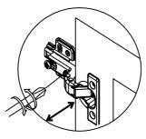
This is used to adjust the door panel in the up and down direction.
