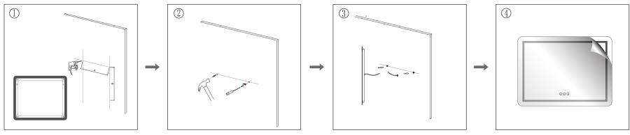
Measure the distance of the mounting hole, Drill holes with a suitable sized drill.
