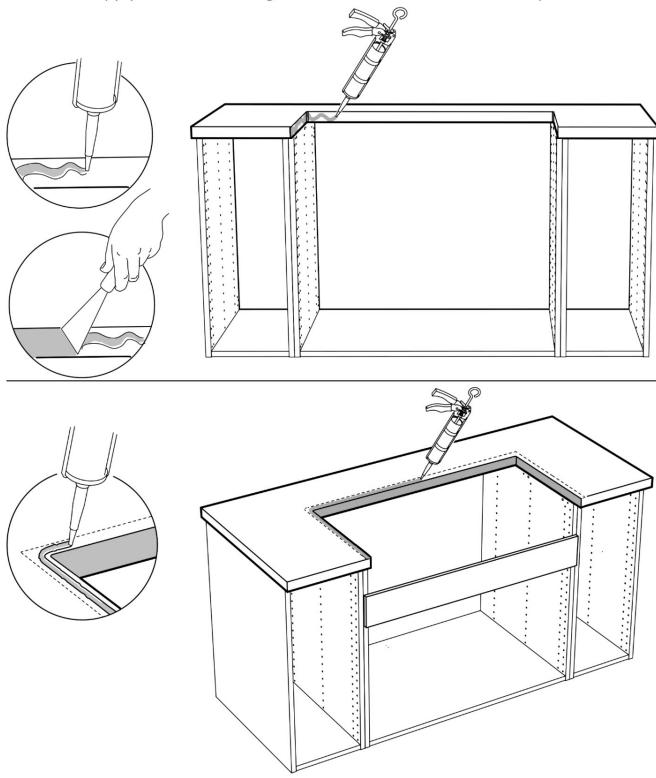
\*IMPORTANT\* To prevent water leaking into the countertop, sink must be installed with all three cut edges sealed with silicone. Silicone is not included.
