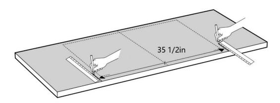
\*IMPORTANT\* Due to the nature of ceramics, each sink dimensions may vary slightly. Make sure your physical sink width is wider than the cut countertop width of 35 1/2in.
