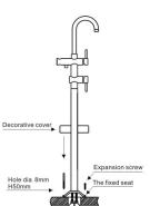
Use the explosion screw to fix the base on the ground, and put the base cover over the base.
