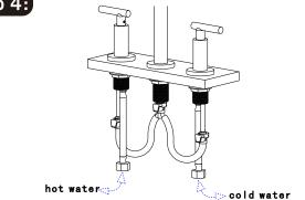
Connect the inlet hoses to the water supply valve. Installation complete.
