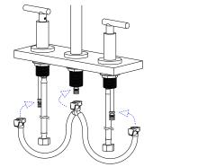
Connect the spout kit and the side body assy with quick connect hose.
