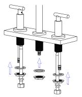
Use the nuts to fix the faucet, gaskets are required between the nuts and the fixing plate.
