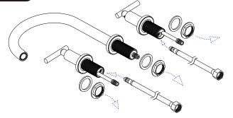
Loosen the nuts and remove the gaskets. Connect the inlet hoses to the side body assy.
