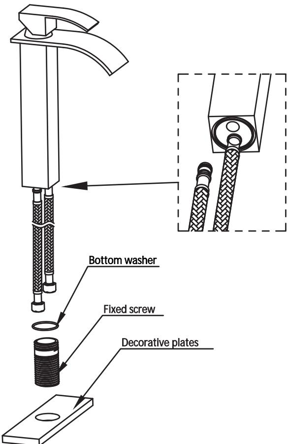
1. Connect the water inlet pipe to the faucet, then put the bottom gasket into the bottom of the faucet, then tighten the faucet with a fixing screw, and then put on the decorative panel.
