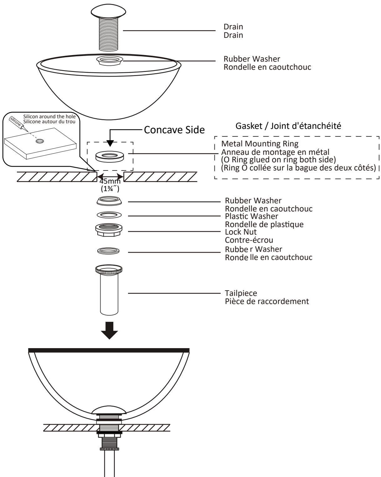
\* ATTENTION : DO NOT OVER-TIGHTEN POP-UP/GASKET WHILE INSTALLING IT TO GLASS VESSEL.
