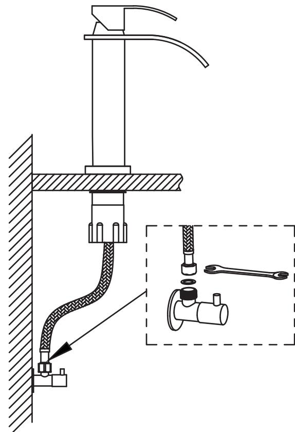
3. Connect the two Inlet pipes on the main body of the faucet to the angle valve. Follow the "red" and "blue" points on the handle of the faucet, the left is red and the right is blue, respectively connecting the "hot"/"cold" water.
