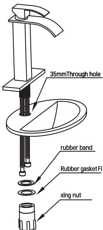
2. Make sure the basin has a 35mm through hole, pass the hose through the hole, pass the rubber ring, rubber washer, and fixing nut into the hose in the order of the drawing, and tighten the fixing nut and the fixing screw to fix the faucet on the basin
