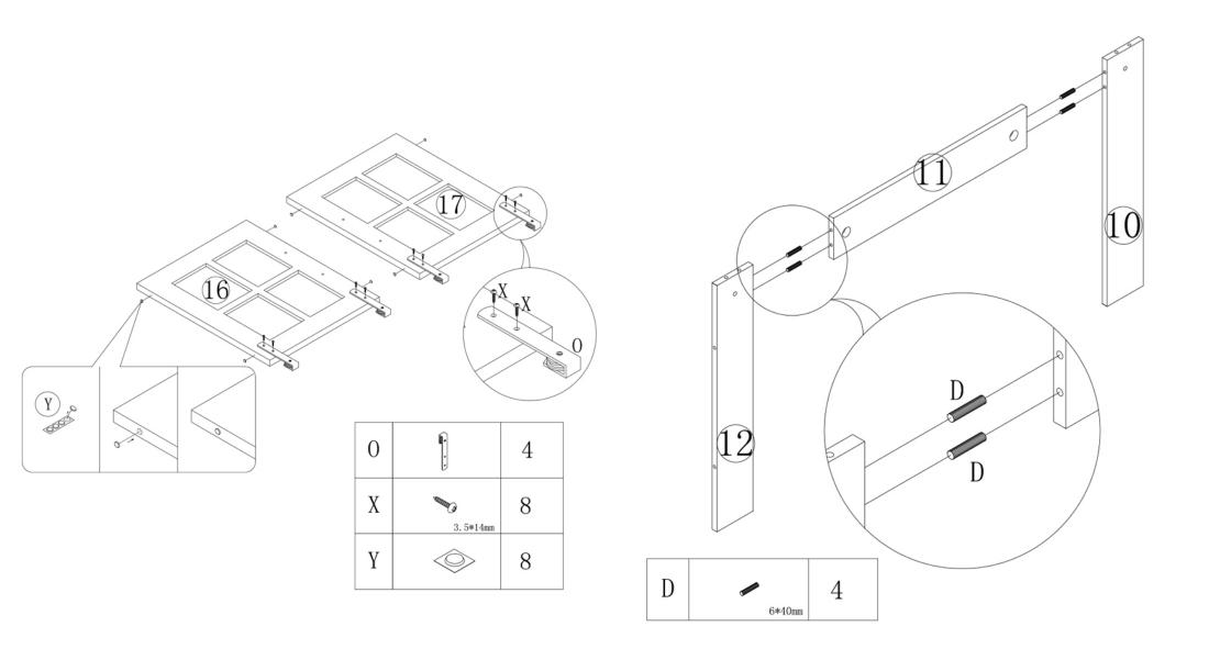
Fix O on Panel 16,17 with Screw X. Stick Y on two sides of Panel 16,17.
