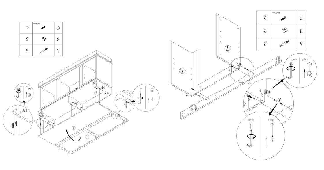
Connect Panel 1 to cabinet body with Camlock A&B and Dowel D.
