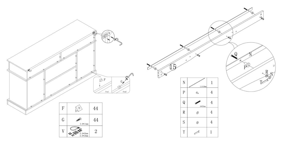
Strengthen the back panel with F by Screw G. Fix V on Panel 1 with screw.
