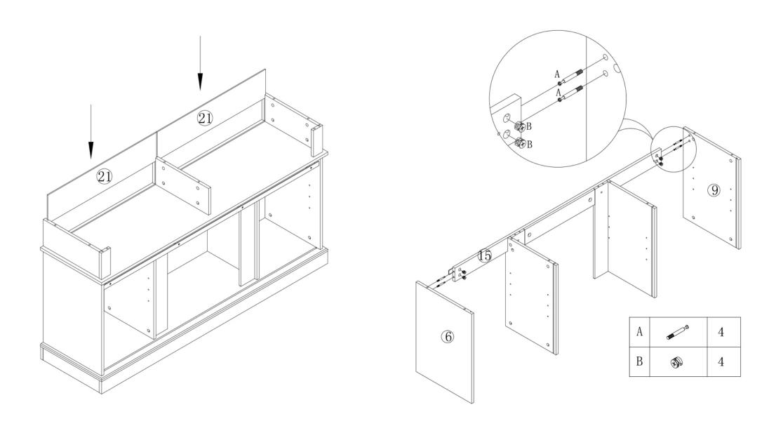
Insert Panel 21 into groove on Panel 4,5.
