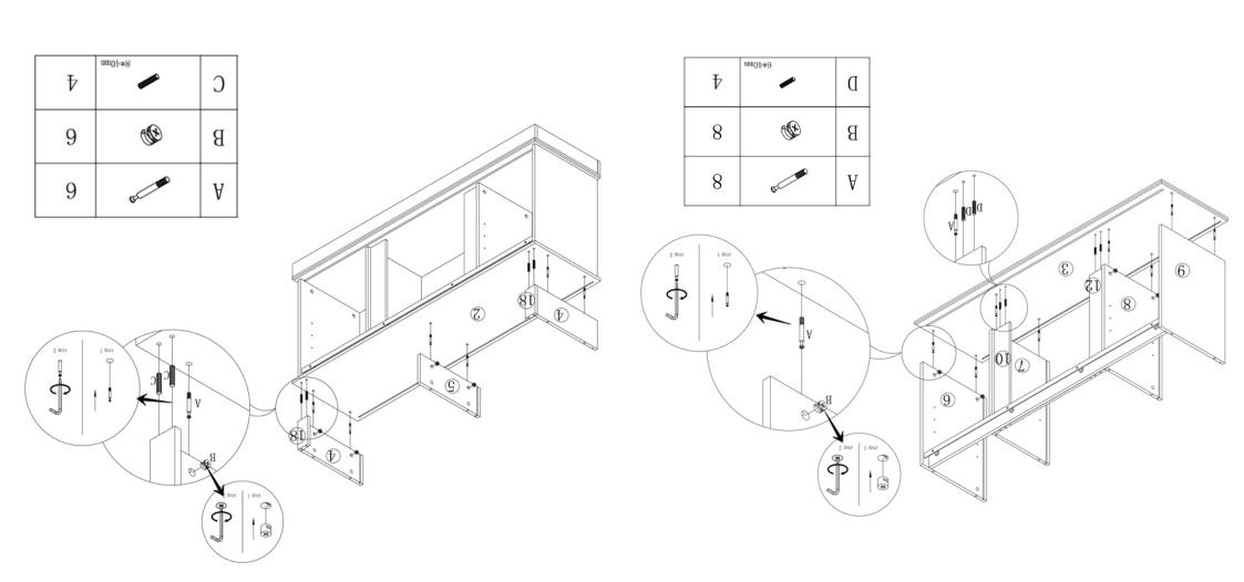
Connect Panel 4,5 to Panel 2 with Camlock A&B. Connect Panel 18 to Panel 2 with Dowel D.
