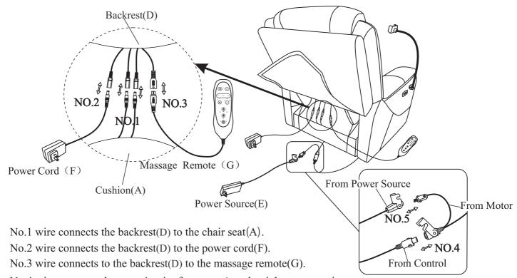
No.4 wire connects the motor's wire from seat A to the right armrest wire connect.
