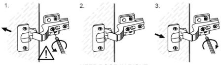
MOVE DOOR OUTWARD by turning this screw counter-clockwise
