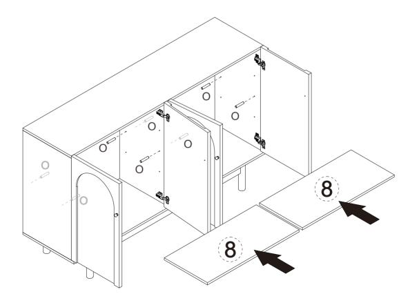
Put hardware O to part 2/3/4 .Put part 8 on hardware O.
