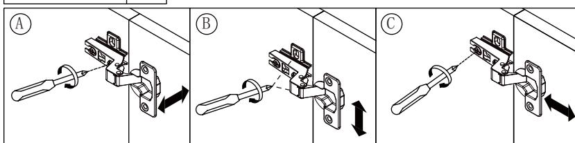
A. Lateral adjustment by screw adjusting
