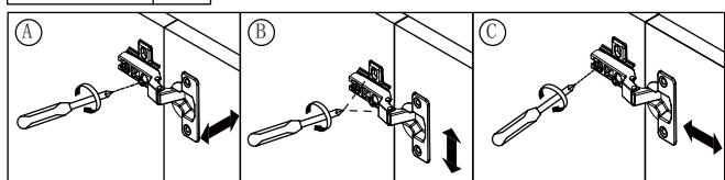
A. Lateral adjustment by screw adjusting    B. Vertical adjustment via slot in the mounting plate    C. Front-to-Back by slackening the hinge arm mounting screw
