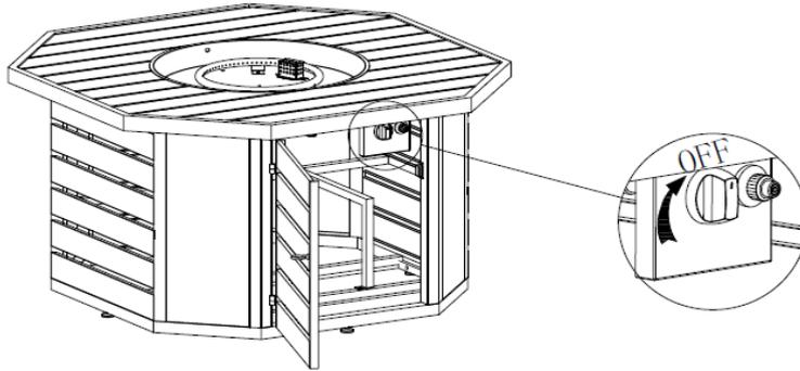
1. Check that the Control Knob (13) for the gas supply system is turned to the "OFF" position before starting any assembly.
