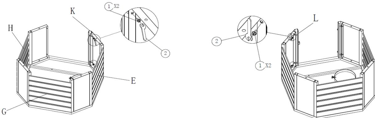
4. Attach door post(K) with panel (F) together using 2pcs of Bolts ① with Allen Key②. Same assembly step for door post(L). Pls do not fully tighten.
