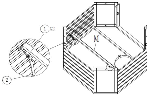
5. Attach stop lever (M) with panel (E) and panel(H) together using 2 pcs of Bolts① with Allen Key②. Pls do not fully tighten.
