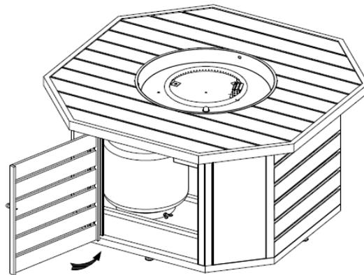
5. Close the Door (C) back to the Mainframe of the Fire Table / Column (C).
