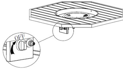
1. Check that the Control Knob (13) for the gas supply system is turned to the "OFF" position before starting any assembly.
