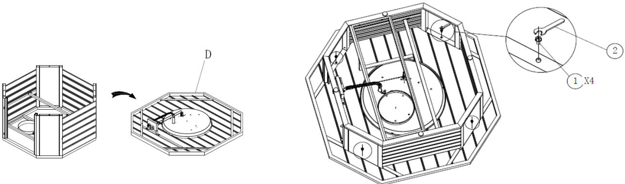
7. Turn over the metal base first and then align it on the table top (D). Fix the metal base with table top (D) using 4 Bolts① with Aleen Key②. And tighten all Bolts.
