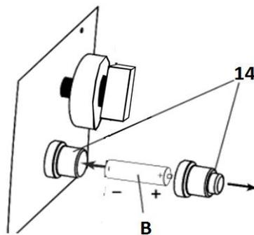
6. Remove the Electronic Igniter Cap (14) on the electronic Igniter (14) by unscrewing and slide the Battery (B) into the battery slot (14). Make sure the positive side of the Battery( B ) faces outwards. Screw the Electronic Igniter Cap (14) over the battery, tightly.
