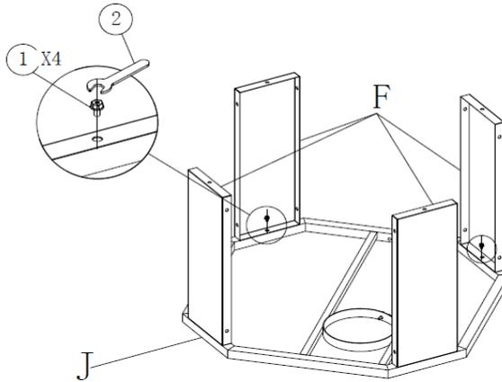
2. Attach panel (F) to metal stand (J) using 4pcs of Bolts①with Allen Key②. Pls do not fully tighten.
