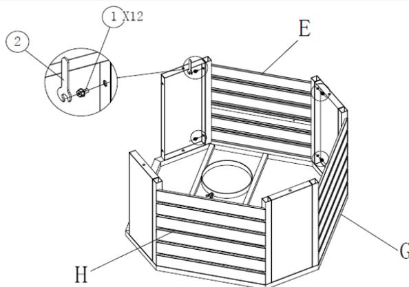
3. Attach panel (E) , panel (G) and panel (H) with panel(F) together using 12pcs of Bolts① with Allen Key②. Pls do not fully tighten.
