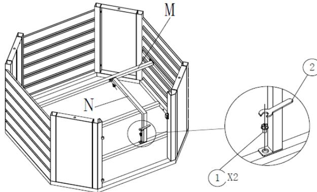
6. Attach stop lever (N) with stop lever (M) and metal stand (J) together using 2 pcs of Bolts①with Allen Key②. Pls do not fully tighten.
