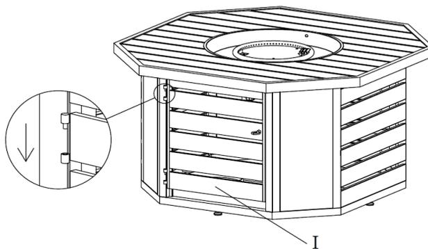
8. Turn over the Gas Fire Table, insert panel with door (I) to the door pivot.
