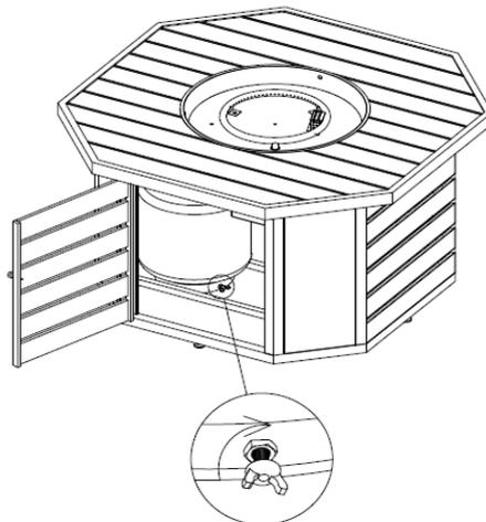
3. Place 20 lb. Propane Gas Tank (not included) into the Metal Stand (18). Make sure the Propane Gas Tank is placed completely into the Metal Stand (18 ). Turn the preassembled Wing Screw (17) in a clockwise direction in to the Nut (17) to secure the Propane Gas Tank tightly.
