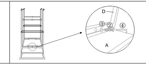
Attach Right Side Panel(D) to the Top Tray(A) through the pipe into the wooden block using Bolt(2) and Washer(3) with Allen Key(4).
