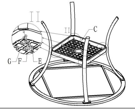
Attach Shelf(C) to Table Legs(B) using Bolt(F) and Flat Washer(G) with Allen Wrench(E).
