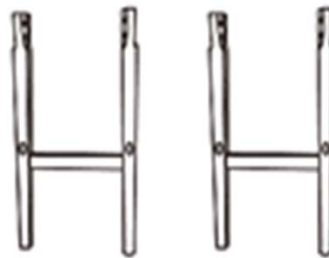
B. 'H' Leg Frames-when assembling, the BOLT points must be INWARD facing.
