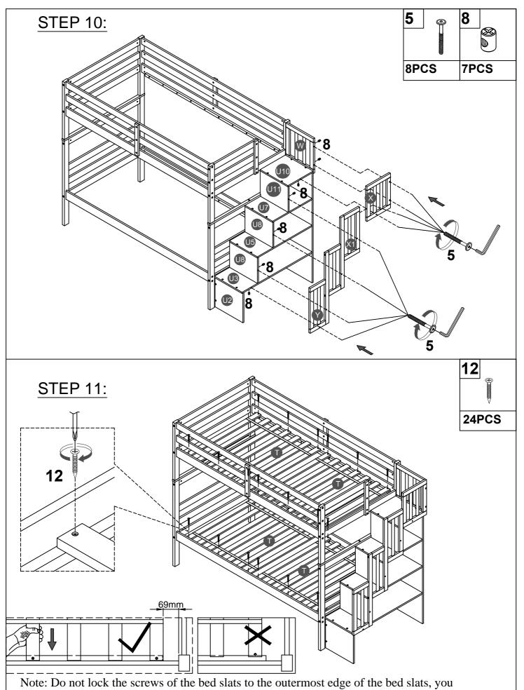
need to leave a certain space at the edges, otherwise it will cause the board to break. Do not lock the bed slats on the edge of the wood, please hold firmly before screwing, hold it in place with one hand, then lock the screw.
