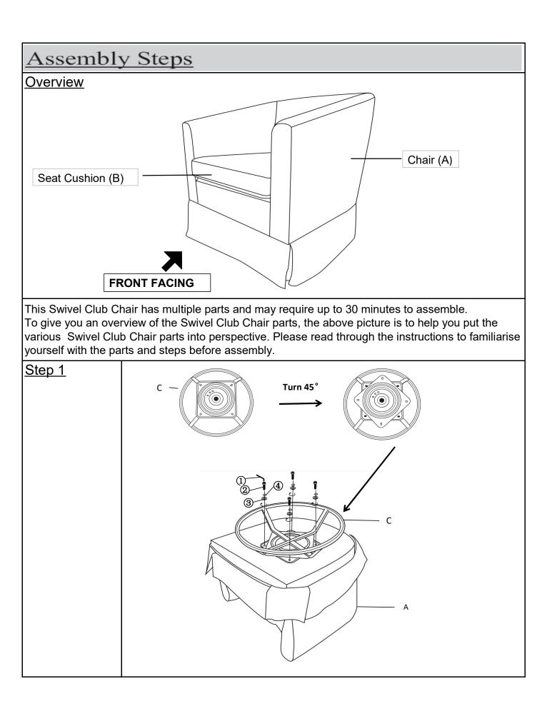
Turn the swivel by 45° first until can see the four mounting positions. Place the Chair(A) face down onto a flat, clean, non-marring surface. Align the Chair(A) to the notch of the Swivel(C) with your partner. Attach the Chair(A) and the Swivel(C) using Bolts(②) and Washer Ring(③) Spring Washer (④) with Allen Wrench(①).
