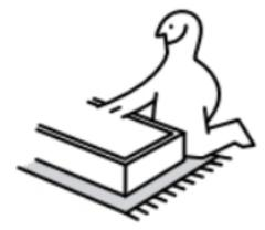
To avoid scratches or damage, assemble the product on a soft surface such as a carpet.
