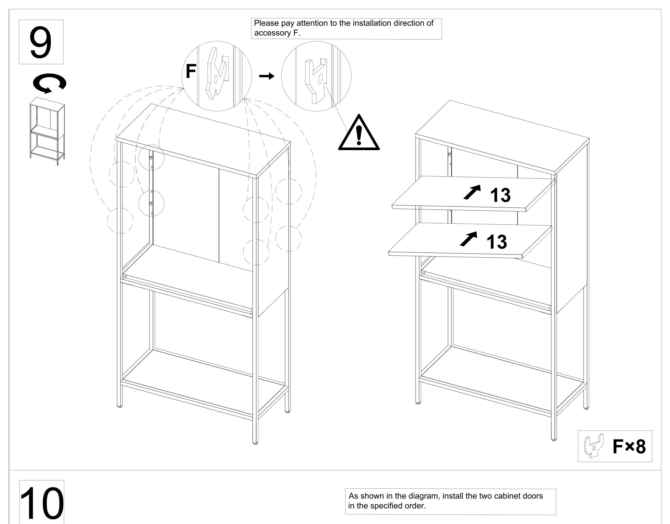
As shown in the diagram, install the two cabinet doors in the specified order.
