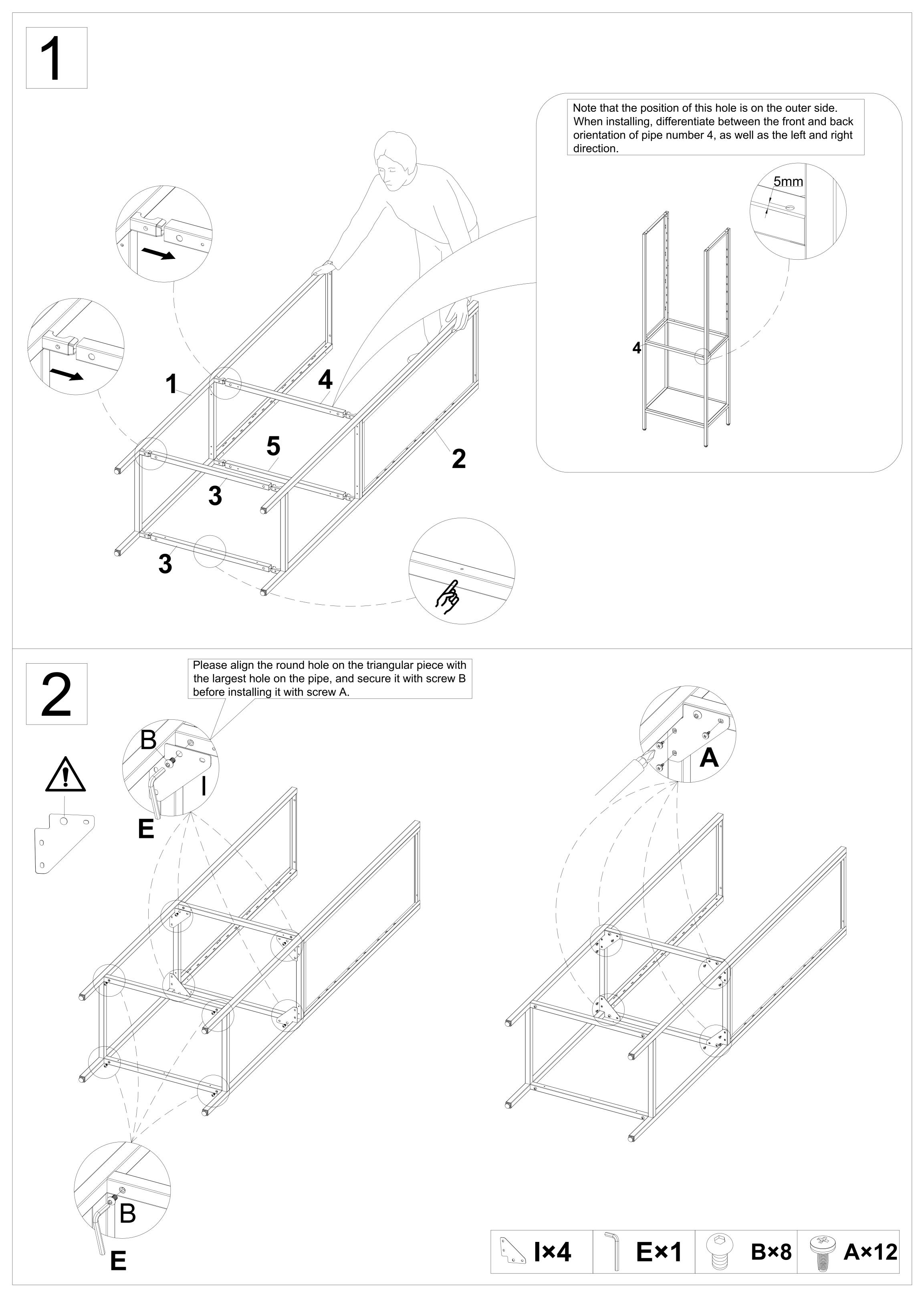
Install component No.6 in the direction shown in the diagram to the specified position, and then secure it in place with screw A.
