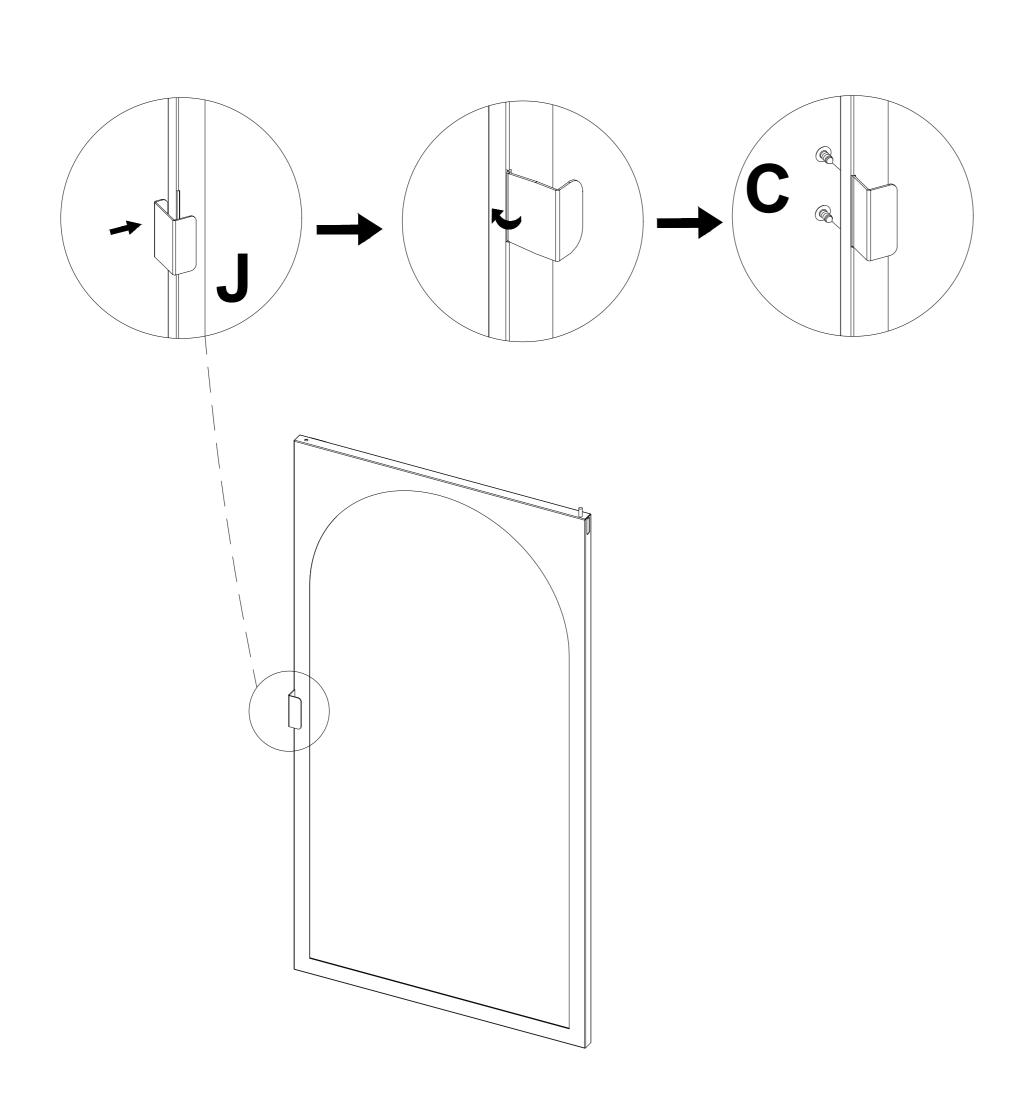
Install the handle in place according to the
