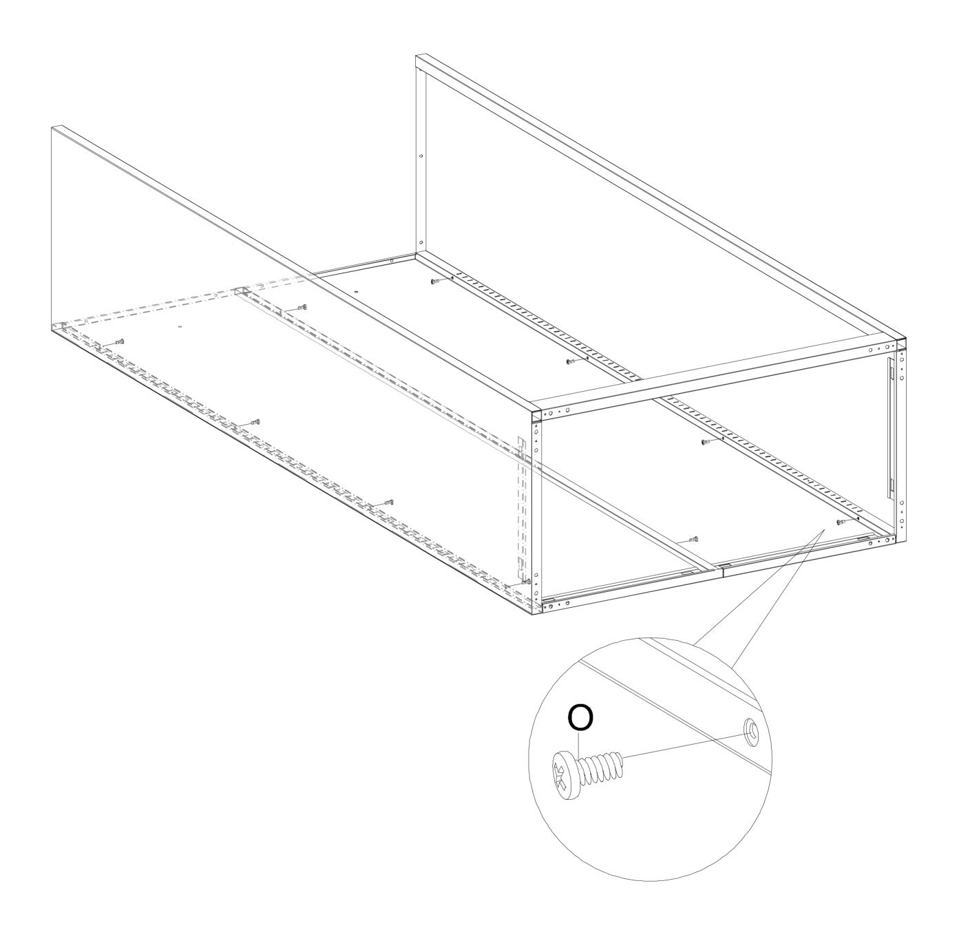
• It is suggested to use an electric drill when installing the screws.
