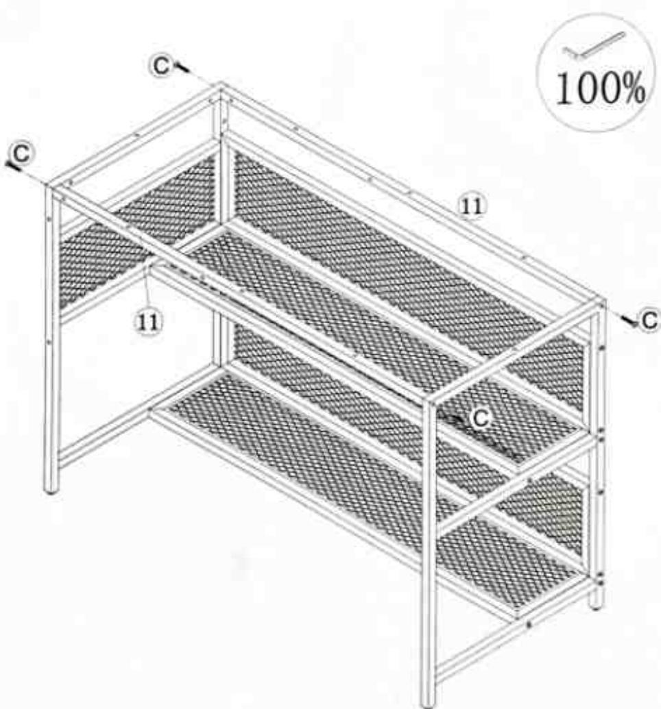
EN-During the assembly, please first half-tighten all the screws into the holes.
