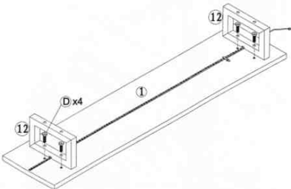
EN-During the assembly, please first half-tighten all the screws into the holes.
