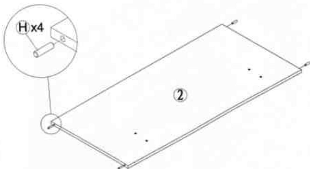
EN-During the assembly, please first half-tighten all the screws into the holes.
