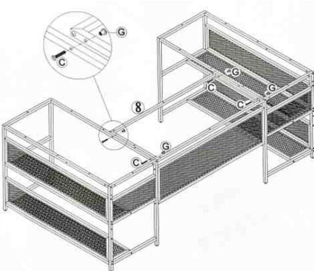
EN-During the assembly, please first half-tighten all the screws into the holes.
