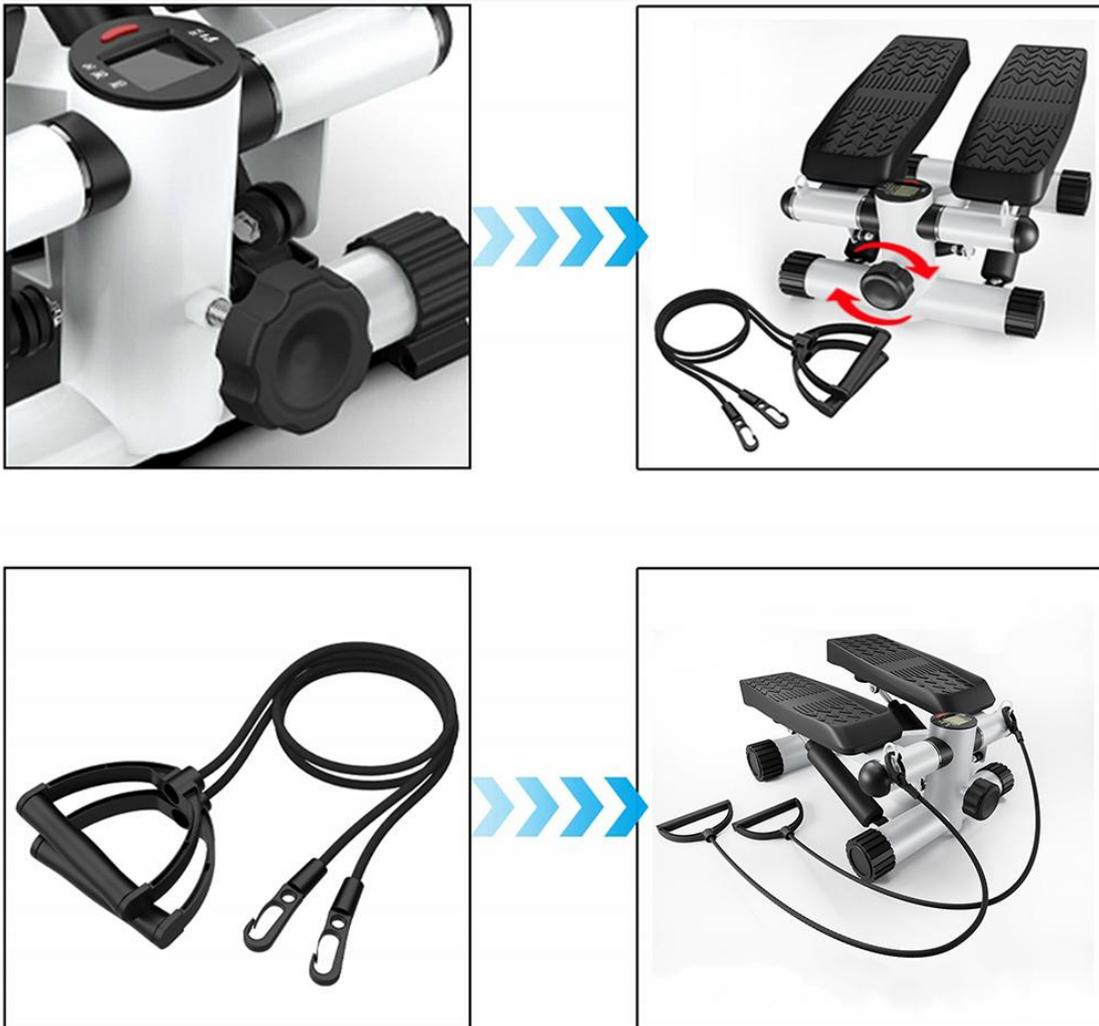
As the picture shows, take out the adjusting button adjust the hole site to the right position, and insert the knob. The knob can adjust the height of the pedal, and the tighter the knob, the higher the pedal.
