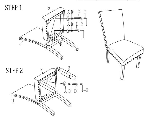
Do not Tighten ANY Bolts Until All Bolts Have Been Started, Stand the chair Upright on Flat Surface. Put Pressure on the chair and Rock it back and forth to adjust to level, Tighten All Bolts With Allen Wrench.
