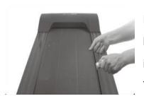
Pull up tightly of the running belt. Then put the silicone oil to running board. Then start the machine to running 3 minutes without loading. It is better to maintain like this every 30 hours working of the machine. This can save lifetime of parts properly.
