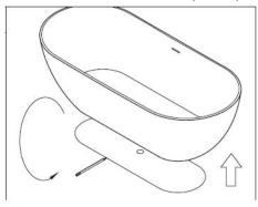
2. Carefully set bathtub into position and rough in your drain pipe (1 1/2") accordingly.
