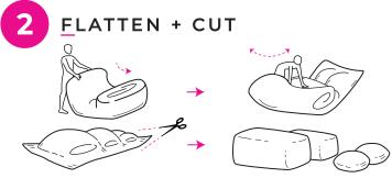
Unfold and flatten the EcoFoam stuffing, then remove the wrapping by cutting it with scissors, revealing four EcoFoam pillows.
