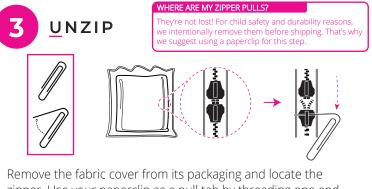
Remove the fabric cover from its packaging and locate the zipper. Use your paperclip as a pull tab by threading one end through the slider body. Set aside the paperclip.
