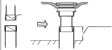
Insert the outlet pipe into the sewer pipe. If the outlet pipe is too short, Please connect it with a tube before inserting. STEP 4
