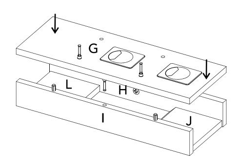
**1** You must drill the bottoms guided by the holes in the structures wiht a 3/16" drill bit.
