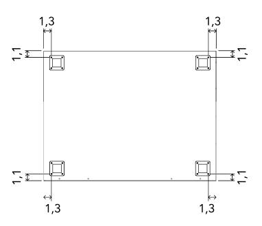
On the piece A measure the points indicated in the diagram, position the legs and secure them with sheet metal screws.
