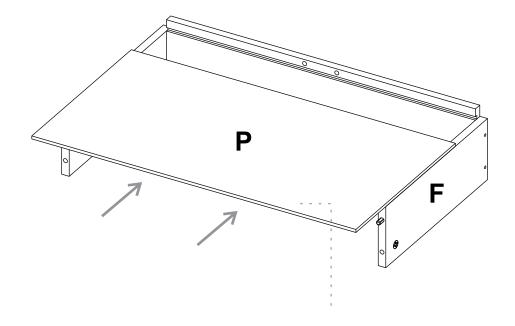
Slide the back panel inside the grooves.
