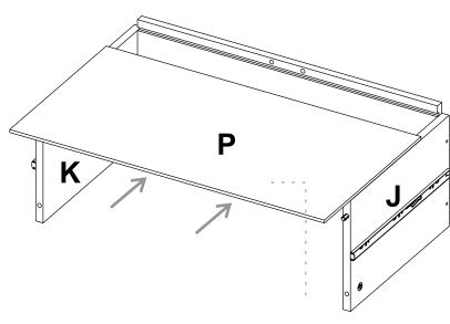
Slide the back panel inside the grooves.
