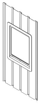
The window set is only used to replace YX- Series metal shed with 156x43cm metal wall panels
