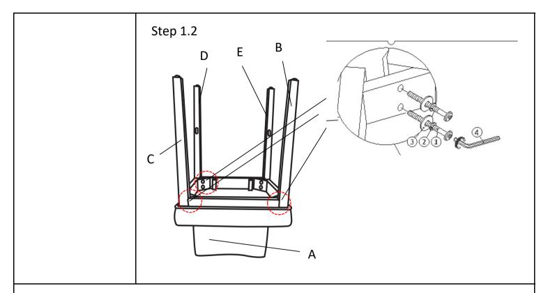
Place the Seat&Back (A), Left Back Leg(E) onto a soft surface to avoid any scratches or damages to the product.
