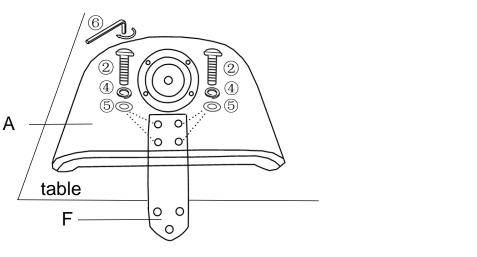
Attach the rectangular end of the Metal Connector (F) onto the Chair Seat (A) as pictured, using the Bolts (2), Spring Washers (4) and Washers (5) with the Allen Key (6).
