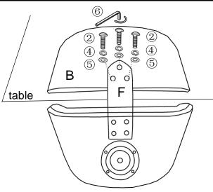
Attach the other end of the Metal Connector (F) onto the Chair Back (B) as pictured, using the Bolts (②), Spring Washers (④) and Washers (⑤) with the Allen Key (⑥). Fully tighten all the Bolts in a sequential manner. Make sure all parts are connected and securely locked into position.
