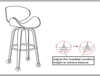
Check the stability and then tighten all the remaining Bolts.
