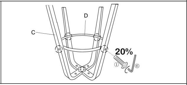
Attach the Footrest (D) to the Legs (C) using the Bolts (1) with the Allen Key (6) as pictured above.
