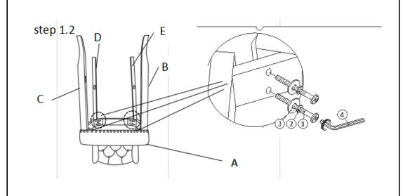
Place the Bar Chair Seat&Back (A), Left Back Leg(E) onto a soft surface to avoid any scratches or damages to the product.
