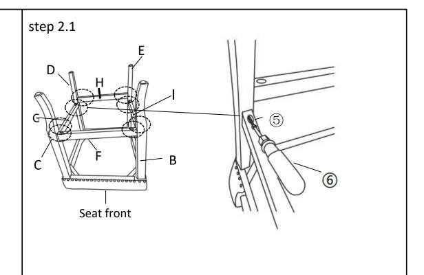
2.1 Insert the Side Rail (G) into round housing of the Legs (D) as shown above.
