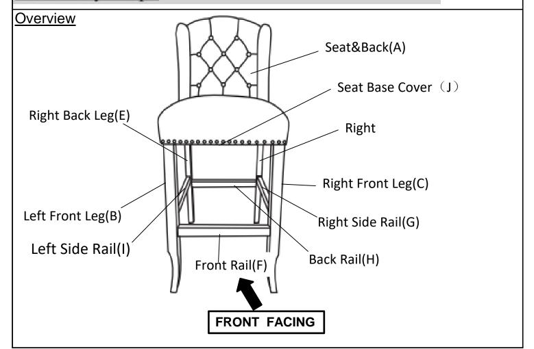
This Bar Chair has multiple parts and may require up to some 30 minutes to assemble. To give you an overview of the barstool parts, the above picture is to help you put the various parts into perspective. Please read through the instructions herebelow to familiarise the parts and steps before assembly.
