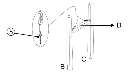
Insert the Short Side Rail (D) into the oval holes of Legs (B,C) forming an 'H' frame by using Screws (5) and Screwdriver as shown above.
