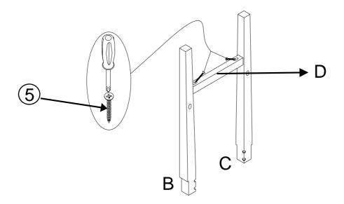
Insert the Short Side Rail (D) into the oval holes of Legs (B,C) forming an 'H' frame by using Screws (⑤) and Screwdriver as shown above.
