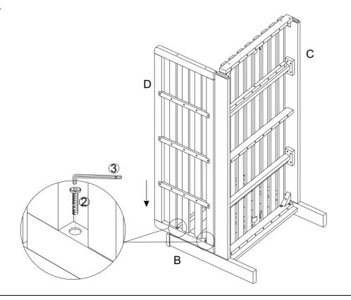
With the help of your adult partner, attach the Backrest (D) to the Right Leg Panel (B) in assemble on step 2 using Bolts (2) and Allen Wrench (3) as shown above. **Do not fully tighten the Bolts.**
