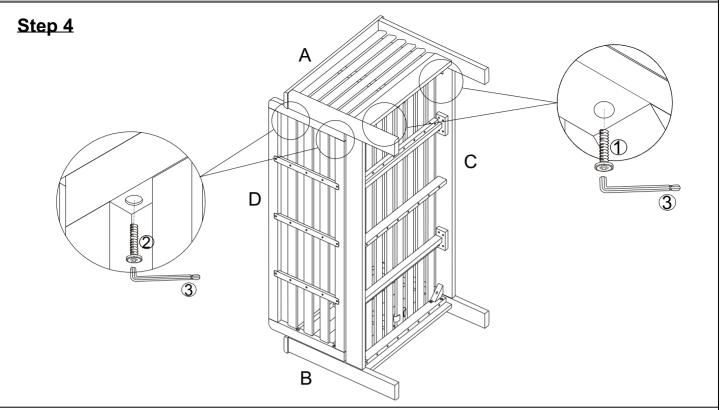
With the help of your adult partner, attach the Left Leg Panel (A) to the Seat Panel (C) and Backrest (D) in assemble on step 3 using Bolts (1), Bolts (2) and Allen Wrench (3). as shown above.
