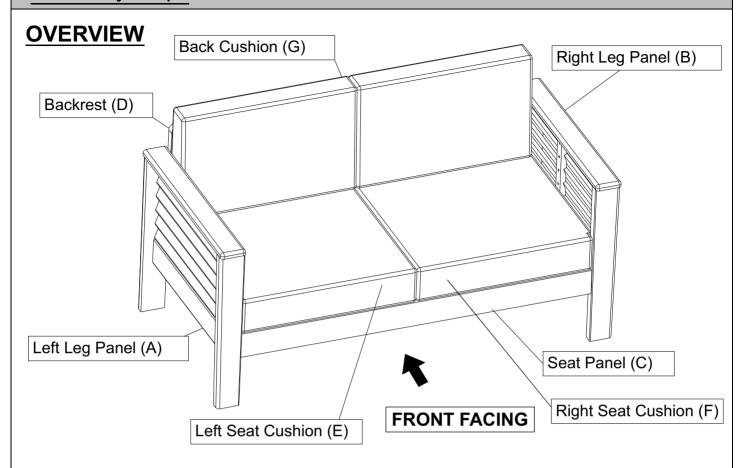
This Loveseat has multiple parts and may require up to 30 minutes to assemble. To give you an overview of the Loveseat parts, the above picture is to help you put the various parts into perspective. Please read through the instructions below to familiarise yourself with the parts and steps before assembly.
