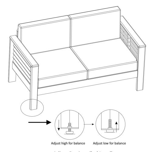
Adjust Pre-installed Levellers high for balance
