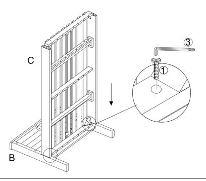
Place the Right Leg Panel (B) on a clean, non-marring surface With the help of your adult partner, attach the Seat Panel (C) to the Right Leg Panel (B) using Bolts(1) and Allen Wrench (3) as shown above. **Do not fully tighten the Bolts.**
