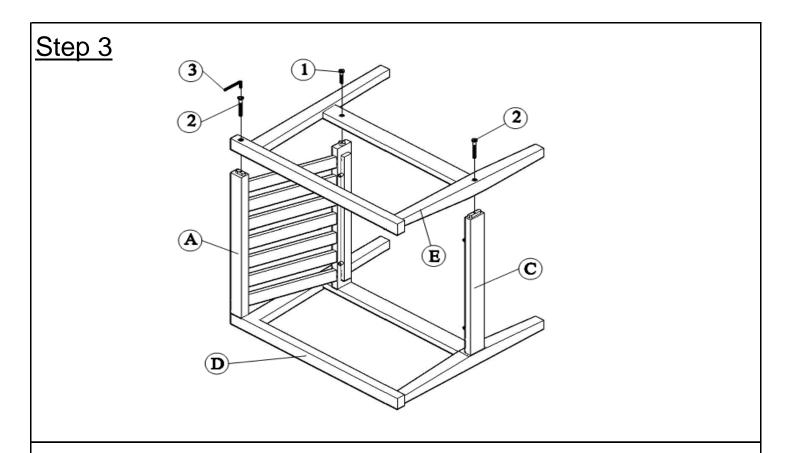
Insert the tenons on Brackrest Panel(A) and Support Bar(C) into mortises of Right Arm Panel(E).
