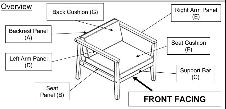
This Chair has multiple parts and may require up to 30 minutes to assemble. To give you an overview of the Chair parts, the above picture is to help you put the various parts into perspective. Please read through the instructions below to familiarise yourself with the parts and steps before assembly.
