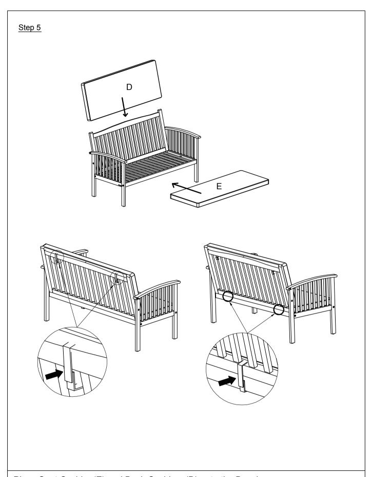
Place Seat Cushion(E) and Back Cushions(D) onto the Bench Tie the magic tape straps of Seat Cushion(E) and Back Cushions(D) to Seat Panel(C) and Backrest Panel(A) as pictured.
