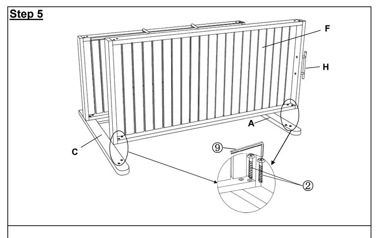
With the help of your partner, align the Top Panel (F) with the holes on the Left Front Leg (A) and Left Back Leg (C) of the assembled part in Step 4, then attach using Bolts ((2)) and the Allen Wrench ((9)) as shown above.
