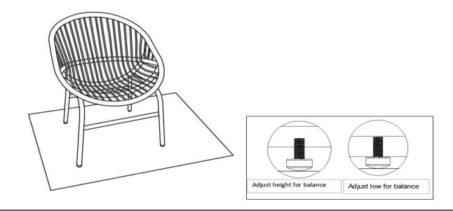
Place the Chair on a LEVEL SURFACE to check for wobbles. Adjust the Leveler to ensure chair stability.
