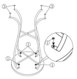
Using Nuts(1) and the Wrench(2), loosely tighten and add Pads(3) onto the feet.
