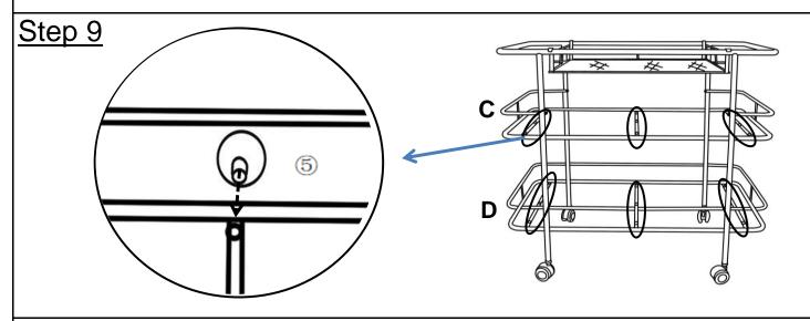
Attach Glass Suction Cups( ⑤) to Middle Shelf Frame(C) and Bottom Frames(D), as shown.
