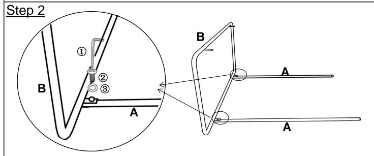
Attach Legs(A) to Top Frame(B) using Bolts(②) and Flat Washer(③) with Allen Wrench(①).
