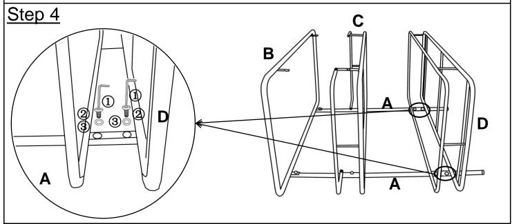
Attach Bottom Frame(D) to Left Frame(A) using Bolts(②) and Flat Washer(③)with Allen Wrench(①).
