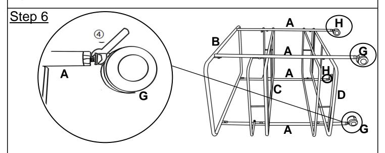
Attach Wheels with Brakes(H) to Legs(A) in Left side using Spanner(4). Attach Wheels(G) to Legs(A) in Right Side using Spanner(4).
