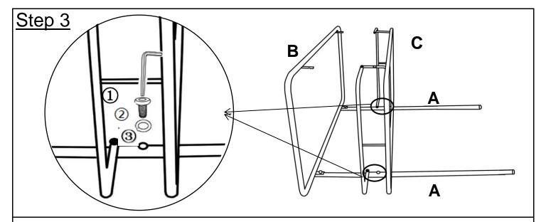
Attach Middle Shelf Frame(C) to Legs(A) using Bolts(②) and Flat Washer(③) with Allen Wrench(①).
