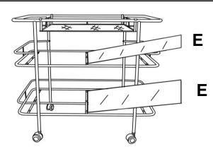
Carefully, insert Glass(E) into Middle Shelf Frame(C) and Bottom Frame(D). Gently press down on the Glass Shelves after you put them into the frame. Please pressure down on each corner to adjust the gap between glass and frame.
