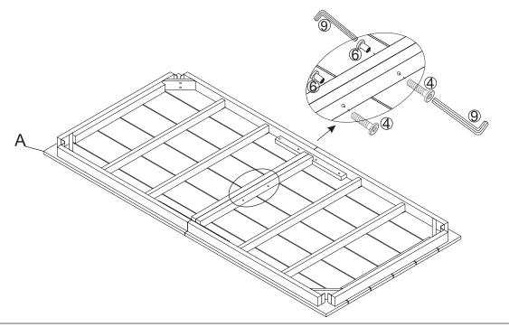
Secure Table Top (A) using the Bolts (4), Sleeve Nut (6) and Allen Wrench (9) as shown in the picture.
