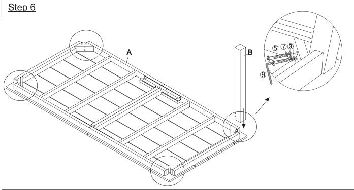
Attach the Legs (B) into the mounting position at the corners of the Table Top (A), using the Bolts (5) with Spring Washers (7), Washers (3) and Allen Wrench(9) as shown in the picture.
