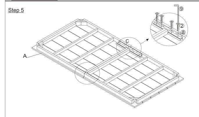
Secure Support Bar (C) to Table Top (A) using the Screws (2), Washer (8) and Allen Wrench (9) as shown in the picture. Repeat the same process with the other Support Bar (C)
