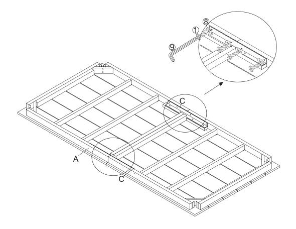
Place Support Bar (C) to the housings of Table Top (A) secure by using the Bolts (1) with Washer (8), and Allen Wrench (9) as show in picture above. Repeat the same process with the other Support Bar (C)
