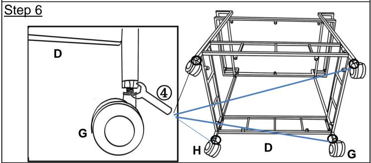
Attach Wheels with Brakes(H) to Left Frame(A) using Spanner(4). Attach Wheels(G) to Right Frame(B) using Spanner(4).
