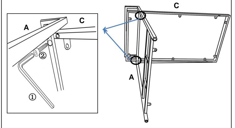
Attach Top Shelf Frame(C) to Left Frame(A) using Bolts(②) with Allen Key(①). **Do not fully tighten the Bolts.**
