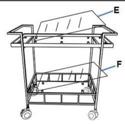
Carefully, insert Top Glass(E) into Top Shelf Frame(C) and Bottom Glass(F) into and Bottom Frame(D).
