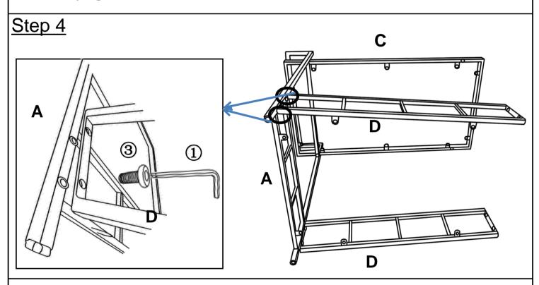
Attach Bottom Frame(D) to Left Frame(A) using Bolts( $\Im$ ) with Allen Key( $\Im$ ). **Do not fully tighten the Bolts.**
